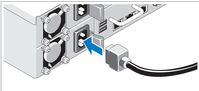
Connect the system's power cable(s) to the system and, if a monitor is used, connect the monitor's power cable to the monitor. Plug the other end of the power cables into a grounded electrical outlet or a separate power source such as an uninterrupted power supply or a power distribution unit.
